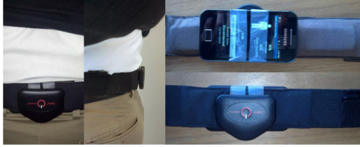
Figure 2: Six Minute Walk Test with Smart Phone Taped to Medical Accelerometer Attached at Stable L3 Point.
